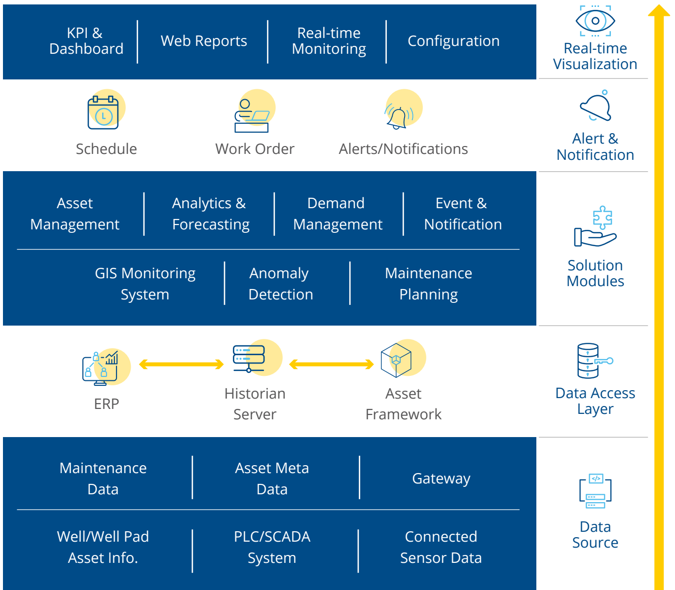
Figure 1: High-Level Solution Architecture
